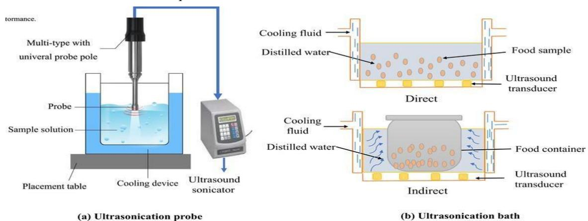
Figure 2.1 Sonication setup (a) shows the layout of a typical sonication process and (b) differentiates between direct and indirect sonication processes.<sup>[4]</sup>
