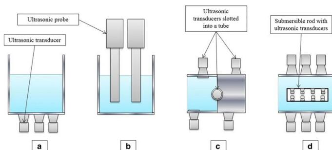
Figure 4.1 Type of ultrasonic reactor designs<sup>[18]</sup>
