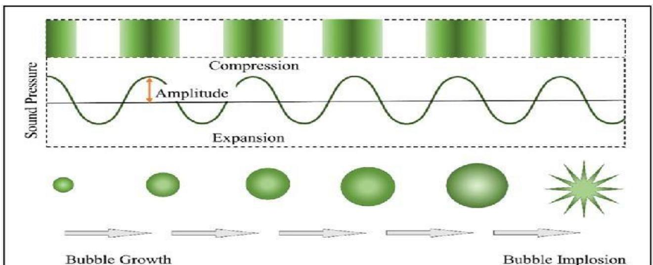
Figure 2.2 depicts the ultrasonication mechanism involving compression and rarefaction cycles.<sup>[3]</sup>
