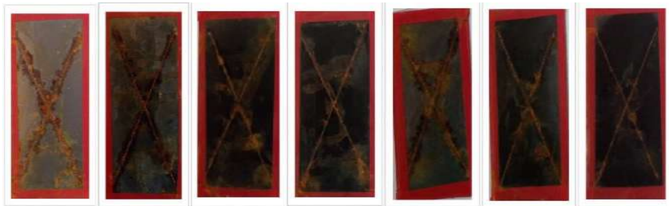
Fig. 4 Panels after exposure to salt spray test (after 1500 hrs)
