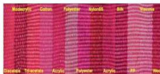
Figure 3: Coloured multifiber fabric with red pigments from Vibrio spp . (Source: Process Biochemistry 48 (2013))
