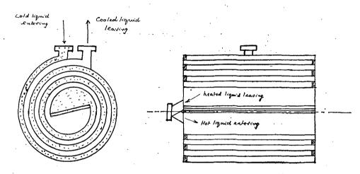
these passages can be of varying dimensions (the passage width may be anything from 3/16 of an inch to one inch) to suit specific flow conditions. Exceptionally long passes obtainable make the spiral heat exchanger suitable for services requiring wide temperature changes and low terminal temperature differences.
