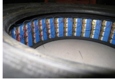
Figure 2- Inner surface of a tyre with an array of lead zirconate titanate benders
