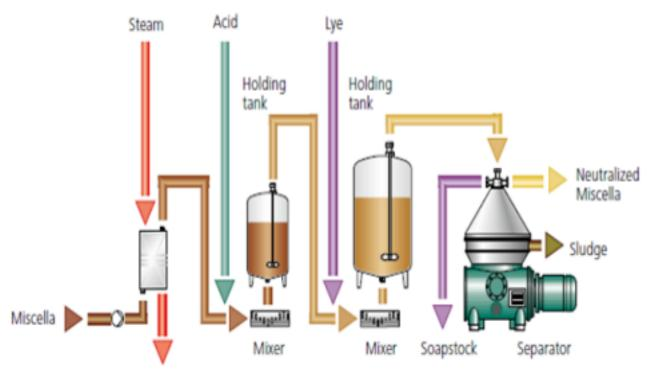
determined by quality and type of oil. This mixture of oil and alkali is transferred from the mixer to a hydration tank and agitated at a slow stirring speed. The is done to improve the hydration of the phospholipids and to coagulate the soaps. The total time required for neutralization is 30 minutes. This coagulated mixture is passed on to the centrifugal separator which separates the mixture into the oil phase and an aqueous phase containing soaps and phospholipids.
