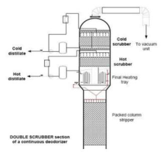
(25)obtained from the deodorizer is accomplished by creating a good contact and heat transfer between the hot vapours and cold distillate, recirculating over the scrubber. There is a packed bed of limited height in the scrubber on which the cold distillate is sprayed. To avoid any carryover of the fatty material to the vacuum system along with the steam, a demister is installed after the scrubber.
