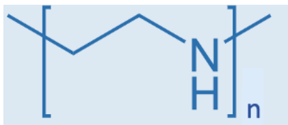
Figure 5: Structure of Polyethyleneimine
